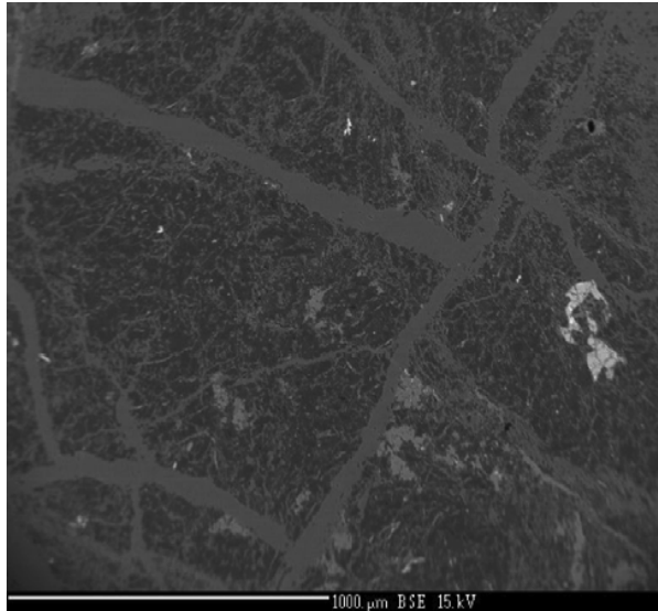
Figure 4: Back-scattered electron image of fully carbonated peridotite (listwanite), composed of magnesite (magnesium carbonate, MgCO_3 , dark grey matrix), quartz (light grey veins showing hierarchical, cross-cutting relationships, filling cracks with spacing < 100 microns) and relict chromian spinel (bright grain at right). Image from keynote talk by Prof. Peter Kelemen, Columbia University, & Streit et al., paper in prep.
